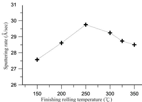
**Fig.6.** Correlation diagram between sputtering rate and finishing rolling temperature of 5N high purity aluminum.
