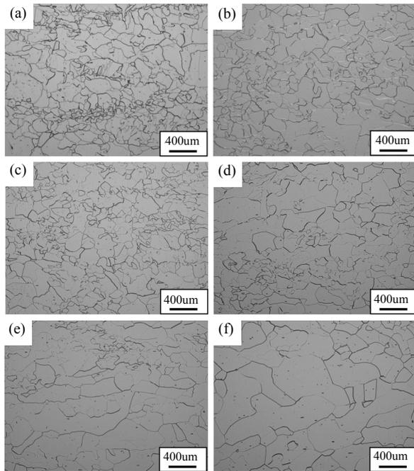
**Fig.1.** OM images of 5N high purity aluminum hot-rolled at various temperature. (a) 150°C, (b) 200°C, (c) 250°C, (d) 300°C, (e) 325°C, (f) 350°C.
