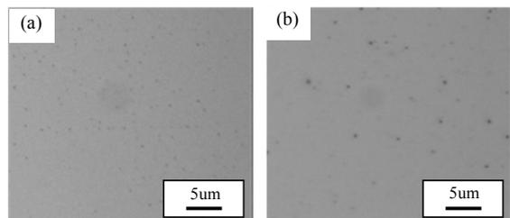
**Fig.10.** OM images of the thin films, sputtered by the 5N high purity aluminum target with sputtering rate  $16.93\text{\AA}/\text{sec}$ , were heat treated at various temperature for 1 minute. (a)  $100^\circ\text{C}$ , (b)  $150^\circ\text{C}$ .
