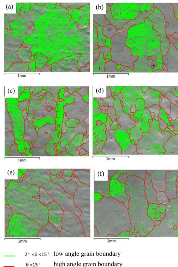
**Fig.3.** EBSD images of 5N high purity aluminum hot-rolled at 250°C, and then heat-treated at various temperature for 1 hour. (a) as-rolled, (b) 100°C, (c) 200°C, (d) 300°C, (e) 400°C, (f) 500°C.
