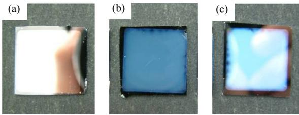
**Fig.11.** The appearance of aluminum thin film which were heat-treated at various temperature for 1 minute. (a) without heat-treatment, (b) 300°C, (c) 400°C.
