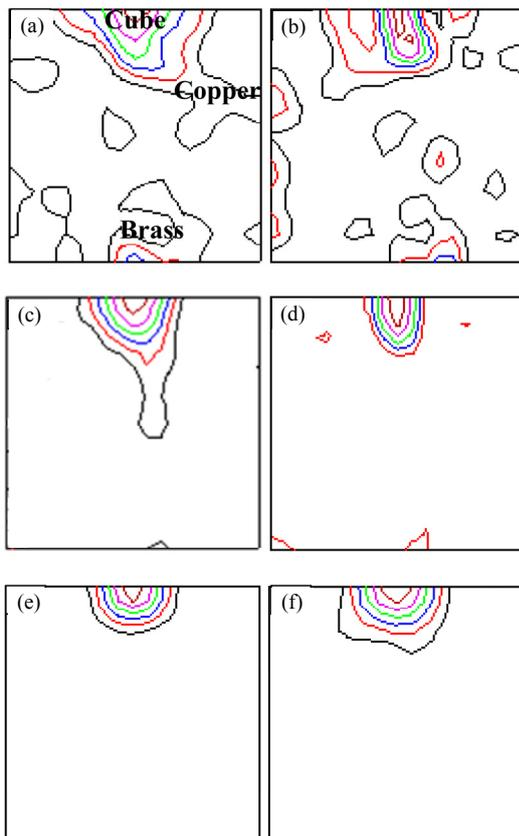
**Fig.4.** The ODFs ( $\Phi_2=45^\circ$ ) of 5N high purity aluminum hot rolled at  $250^\circ\text{C}$ , and then heat-treated at various temperature for 1 hour. (a) as-rolled, (b)  $100^\circ\text{C}$ , (c)  $200^\circ\text{C}$ , (d)  $300^\circ\text{C}$ , (e)  $400^\circ\text{C}$ , (f)  $500^\circ\text{C}$ .
