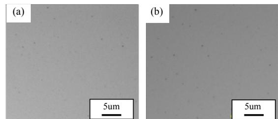
**Fig.9.** OM images of the thin films, sputtered by the 5N high purity aluminum target with sputtering rate  $27.57\text{\AA}/\text{sec}$ , were heat treated at various temperature for 1 minute. (a)  $150^\circ\text{C}$ , (b)  $180^\circ\text{C}$ .
