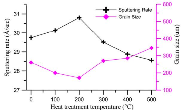
**Fig.7.** Correlation diagram between sputtering rate, heat-treatment temperature and grain size of 5N high purity aluminum hot-rolled at 250°C.
