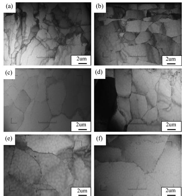
**Fig.5.** TEM images of 5N high purity aluminum hot-rolled at  $250^\circ\text{C}$ , and then heat-treated at various temperature for 1 hour. (a) as-rolled, (b)  $100^\circ\text{C}$ , (c)  $200^\circ\text{C}$ , (d)  $300^\circ\text{C}$ , (e)  $400^\circ\text{C}$ , (f)  $500^\circ\text{C}$ .
