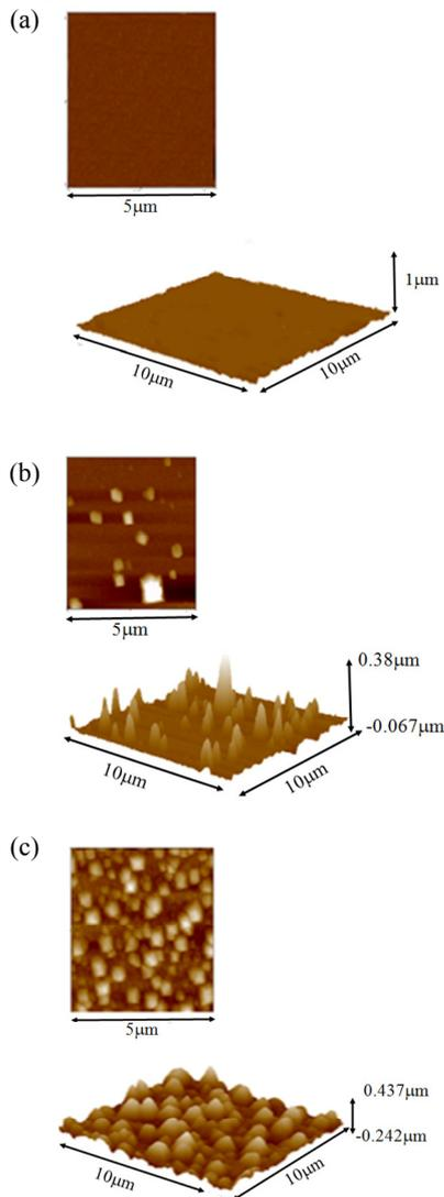
**Fig.12.** The AFM observations of aluminum thin film which were heat-treated at various temperature for 1 minute. (a) without heat-treatment, (b) 300°C, (c) 400°C.
