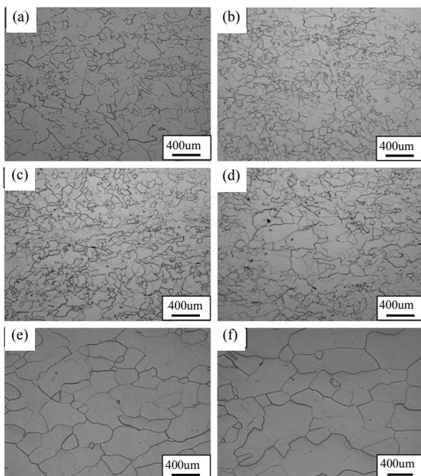
**Fig.2.** OM images of 5N high purity aluminum hot-rolled at 250°C, and then heat-treated at various temperature for 1 hour. (a) as-rolled, (b) 100°C, (c) 200°C, (d) 300°C, (e) 400°C, (f) 500°C.
