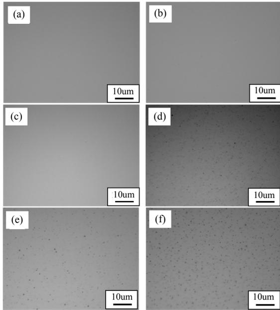
**Fig.8.** OM images of the thin films, sputtered by the 5N high purity aluminum target with sputtering rate  $29.75\text{\AA}/\text{sec}$ , were heat treated at various temperature for 1 minute. (a) without heat-treatment, (b)  $150^\circ\text{C}$ , (c)  $200^\circ\text{C}$ , (d)  $250^\circ\text{C}$ , (e)  $300^\circ\text{C}$ , (f)  $400^\circ\text{C}$ .
